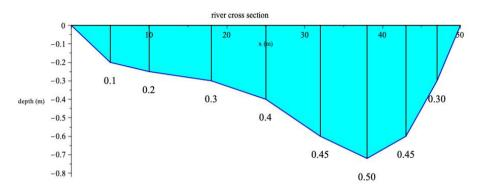
Depth d(x) m for  $a \le x \le b$ . Velocity v(x) m/s for  $a \le x \le b$ . Flow  $\int_{a}^{b} v(x)d(x)dx$   $m^3/s$ .
